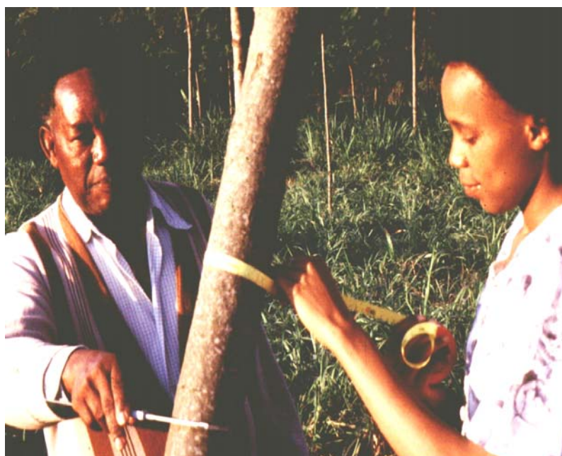
Measuring tree diameter with a diameter tape (above, left) and calipers (below, right).
