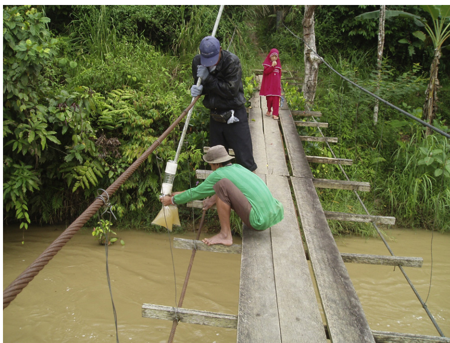
Fig. 2. Collection of depth-integrated runoff and suspended sediment samples at Talang Nangka (WB8).
