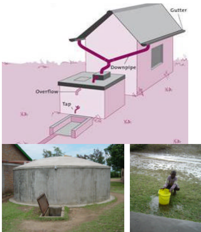
Figure 22 Rooftop rainwater harvesting
