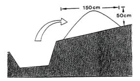
Figure 4-2: Construction of the fanya juu terrace<sup>20</sup>
