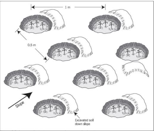
Figure 5-2: Layout of zai pits constructed on a gentle slope<sup>17</sup>.
