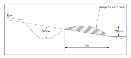
Figure 3-2: Cross section of a contour bund<sup>14</sup>
