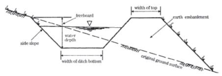
Figure 12-2: Cross section of a trapezoidal cut-off drain<sup>43</sup>
