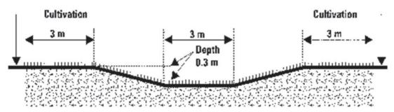
Figure 10-2: Cross-section of a typical grassed waterway<sup>37</sup>
