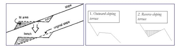
*a)* The cut and fill procedure used to construct bench terraces (b) Types of bench terraces in cross section
