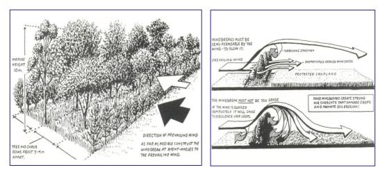
Figure 16-2: a) An illustration of a multi-storey windbreak b) Windbreak design44
