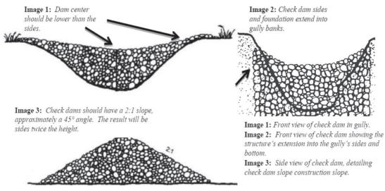
Figure 2-2: A stone check dam profile9
