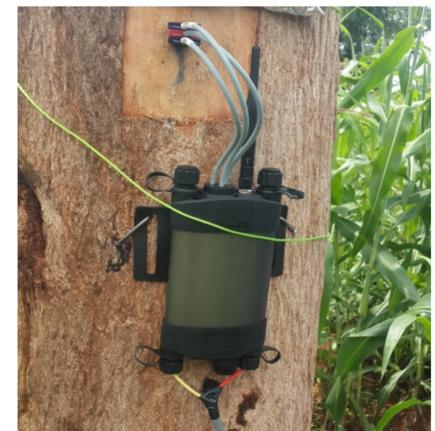
Sap Flow Meter installed in *G. robusta* tree
