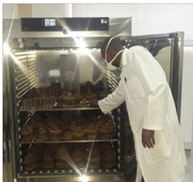
Methods used for the estimation of tree biomass including standing tree measurements (A); destructive sampling for tree biomass partitioning (B) and determination of oven-dry weight of tree biomass samples (C)
